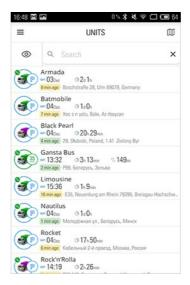
The work list contains dynamically updated unit information. This information includes current moving state, data actuality, state beginning time, duration, and address. Note that address information can be substituted by unit's presence in geofences. To do so, activate *Geofences as addresses* checkbox in the *Other* section of the Wialon Mobile Client settings.
